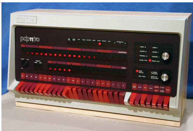
Fig. 2 - The computer PDP-11
